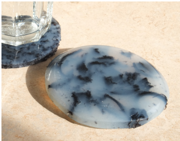
Bioplastic composite with fabric scraps as reinforcement
